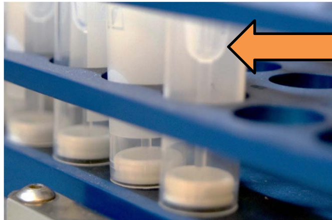
Robot draws from bottom / no dead volume
