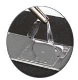
Uses CytoBond Removable Coverslip Sealant that removes easily and cleanly in one piece post-hybridization.
