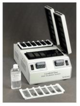
Dual temperature slide heating instrument for performing denaturation and incubation of FISH slides. Consists of two independently controlled heat blocks that each hold a removable 6-slide tray. Trays streamline slide set up and are used to transfer slides between the heat blocks. A built-in temperature calibration system eliminates the cost of third party calibration required for CLIA compliance.
