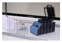
The NoZone WS Workspace features a flexible curtain to allow for manual processing of up to 16 arrays with the Hybex<sup>®</sup> Microarray Incubation System.
