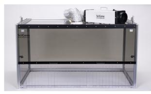
Bench top enclosure with external high efficiency ozone filtration system that provides a clean, ozone-safe, low light workspace for microarray work. Use with the Little Dipper Processor or for manual sample preparation and slide processing. Maintains an ozone level below 5 parts per billion (ppb).
